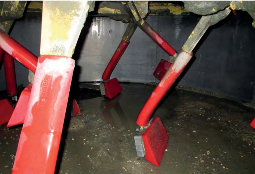
Figure 11: Paddles, arms, and side scrapers are protected by user-replaceable polyethylene guards that extend the life of mixer parts and liner. Automatic washout system uses 3D water jet geometry to reach all areas of the mixer interior, removing most concrete build-up.
