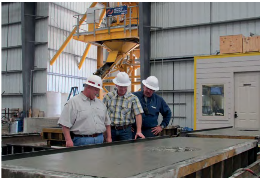
Figure 15: Capital Precast general manager Chad Holden (left), founder and president Ash Wineinger (center) and plant manager Joe Deal, inspect a freshly poured storm water inlet top. The new batching system (in background) provides consistent, high quality SCC for fast pours with no vibration required.
