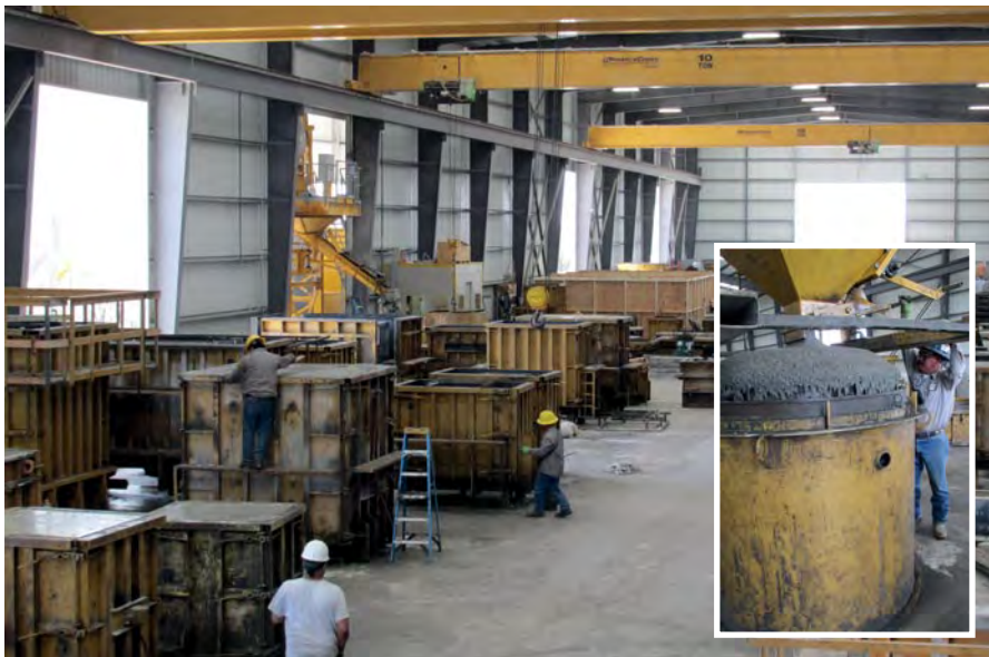
Figure 4: Inside view. The centrally located ACT MobilMat Mo3450-4-PCS (left) supplies SCC mix to all areas of the 50,000 s.f. production floor via several overhead bridge cranes equipped with multiple crane buckets.
