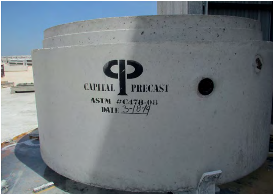
Figure 3: A large manhole base is ready for yarding. Consistent, high quality SCC provides high quality finish and the highest possible strength with lower overall production cost.
