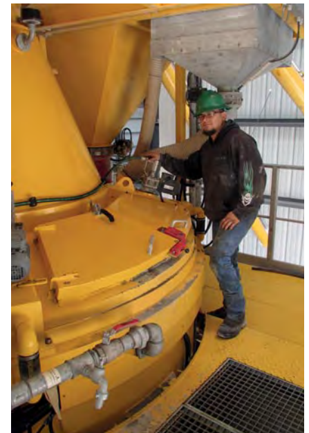
Figure 5: Capital Precast plant operator Daniel Ybanez stands on the mixer platform of the plant's new MobilMat batching system. The Wiggert HPGM 3450 planetary counter-current mixer uses three high speed mixing stars equipped with a total of nine paddles to deliver three cubic yards of consistent SCC mix every few minutes. An automatic mixer cleaning system uses motorized rotating nozzles and high pressure water to clean the mixer in about 10 minutes.
