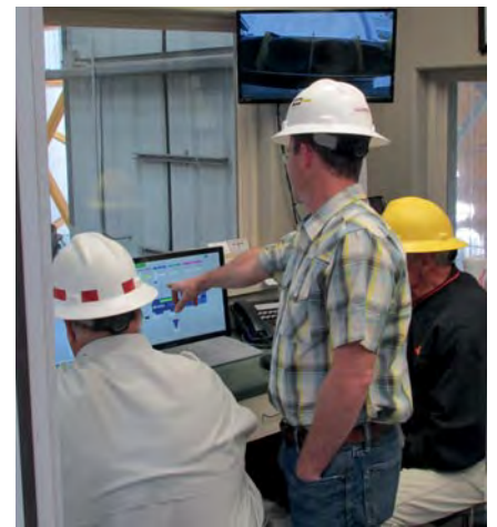
Figure 10: The Capital Precast team checks batching operation statistics in the control room located on the production floor. The PCS Control integrates all batching systems and provides point-and-click ease of use. Recipe recall, material inventory tracking, batching history, maintenance scheduling, and much more are provided by the PC-based control system.
